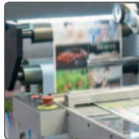
Offset printing stands out by using primarily CMYK process colors with screen rulings from 150 lpi up to 300 lpi. Additionally, offset printing products are typically produced in quite high volumes.
