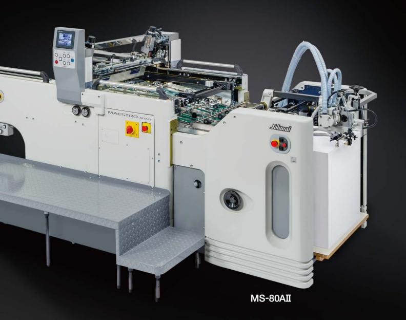
The combination of high precision and productivity - Fully Automatic Ultra-High Precision Rotary, Stop Cylinder Screen Press
