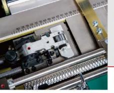
Bearing type side register system is applied. (MS102AX: Pull/push type, MS80All: Pull type) Cylinder built-in front master frame carrier to hold the aluminum screen frame in cams, and a two-step action cam helps reduce the lay sensors and side lay sensors are in standard so the position instantly and securely. Fine registration can be
